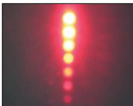
Fig. 1. The pattern observed on the screen due to a laser beam reflected from a glass mirror.
